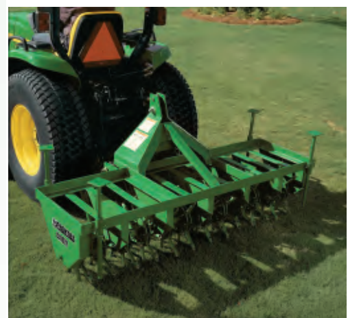
Part of Spring cleanup is Aeration which allows more nutrients, air and water into the root system.
